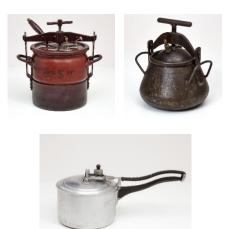
The doctor Denis Papin was fascinated by steam pistons and invented the safety valve in 1679. He decided to fit it into his famous meat-cooking machine known as the digester. The machine uses steam placed under pressure in a closed container, allowing the boiling point of water to be raised to 140°C. This system means you can save energy, have a shorter cooking time and retain more of the vitamins and minerals.
